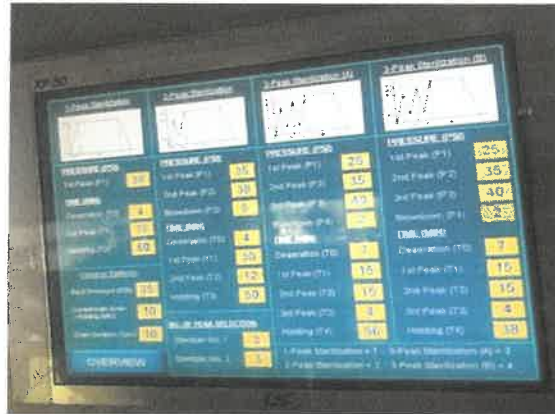
Screen Showing the Sterilization Process (Pressure and Time)
