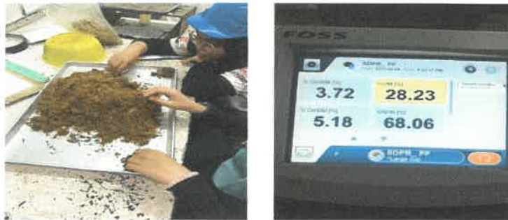
Broken Nut Analysis and Oil Loss Test
