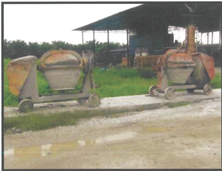
Photo 3.21: concrete mixer to mix the cement
