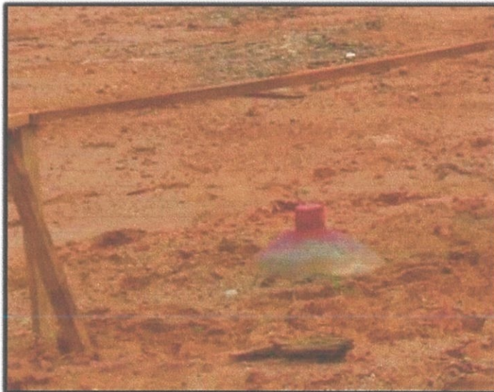
Photo 3.3: stone and concrete for marked the point centre, Sabak Bernam Selangor
