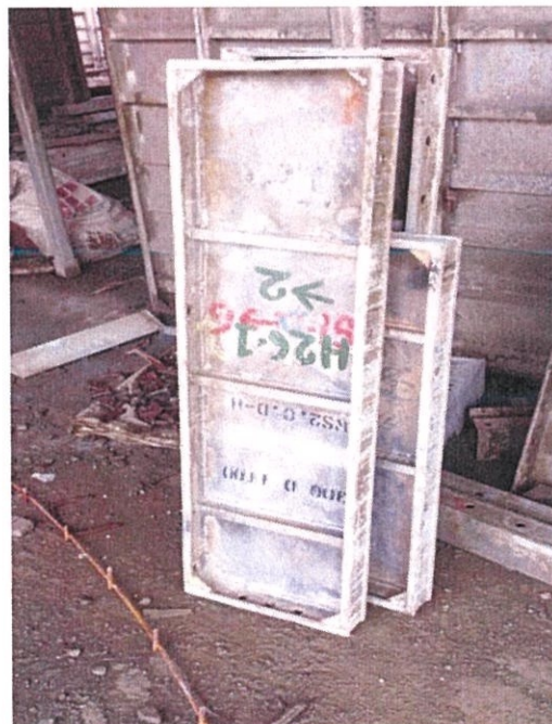
Photo 3.12: Beam Side Panel
