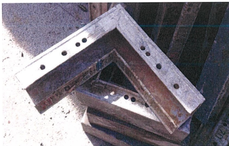
Photo 3.33: Internal Soffit Corner
