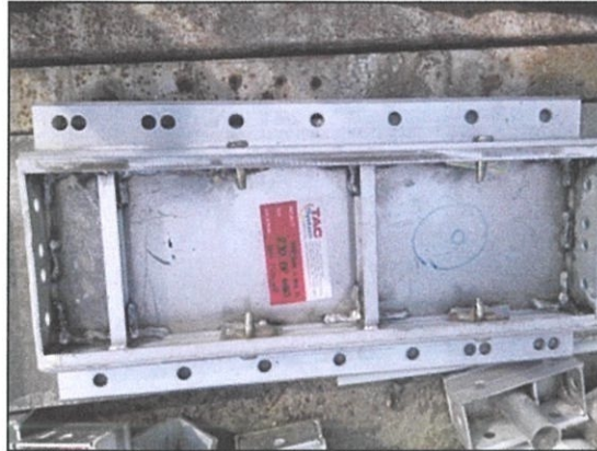
Photo 3.16: Beam Panel (BP)
