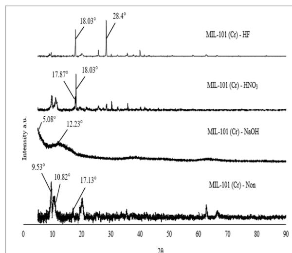
Fig 2: XRD patterns of MIL-101(Cr)–Non, MIL-101(Cr)–NaOH, MIL-101(Cr)– $\text{HNO}_3$ , and MIL-101(Cr)–HF
