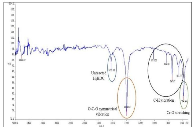
Fig 5: FTIR plot of MIL-101(Cr) – HNO<sub>3</sub>
