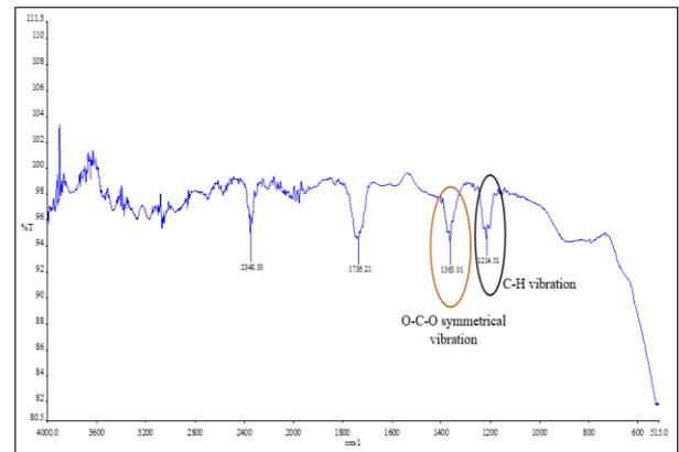
Fig 4: FTIR plot of MIL-101(Cr) – NaOH
