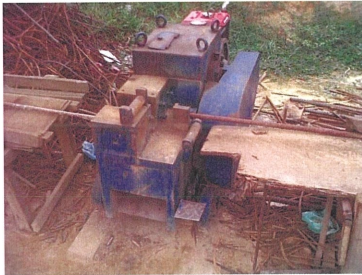
Photo 3.4.2 Bar cutter machine that use in construction of concrete dome structure
