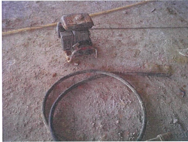
Photo 3.4.3 Vibrator machine that use during concrete work
