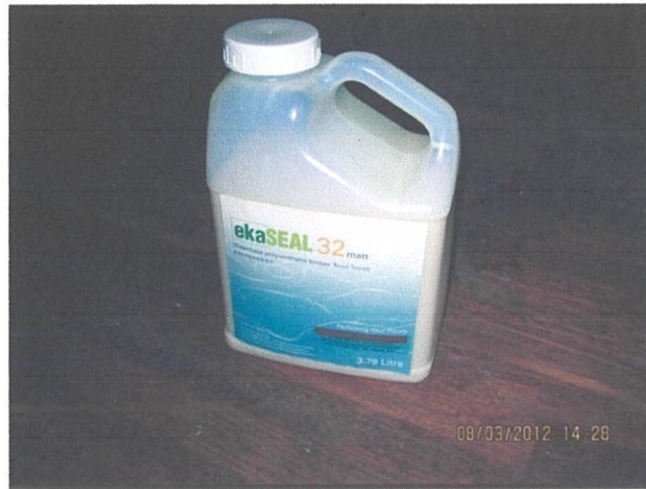
Gambar 3.48 Water base polyurethena Foto Kredit: Asrul Asari (8 Mac 2012).
