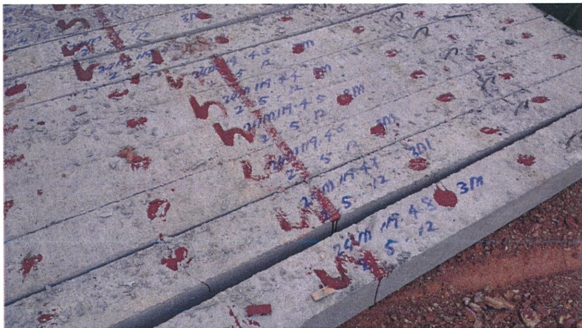
Photo 3.2 The 150mm X 150mm X 3m Piles.
