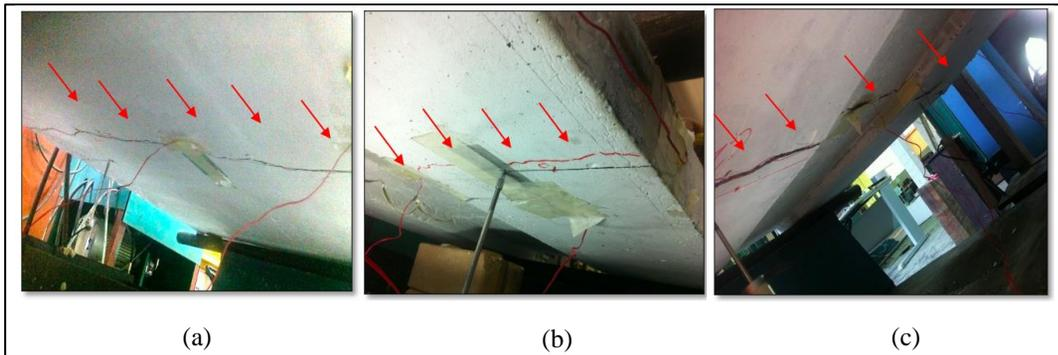
**Figure 7:** Mode of failure of all samples; (a) solid-SFRC, (b) rib-SFRC, (c) rib-SFRC-GFRP
