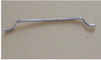
**Figure 2:** Hooked-end steel fibres
