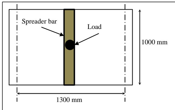
**Figure 2:** The plan view of SFRC Solid and Two Ribbed Slab
