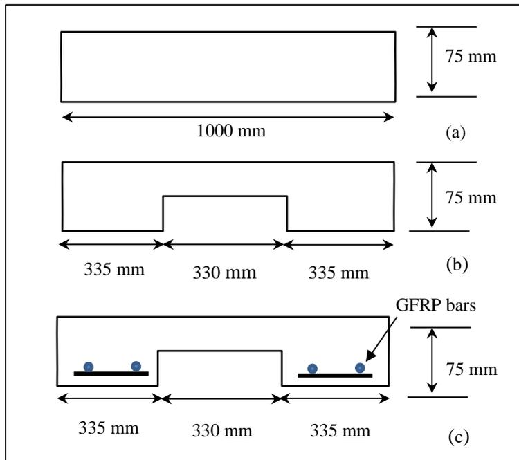
**Figure 3:** The cross section of (a) solid-SF (b) rib-SF and (c) rib-SF-GFRP
