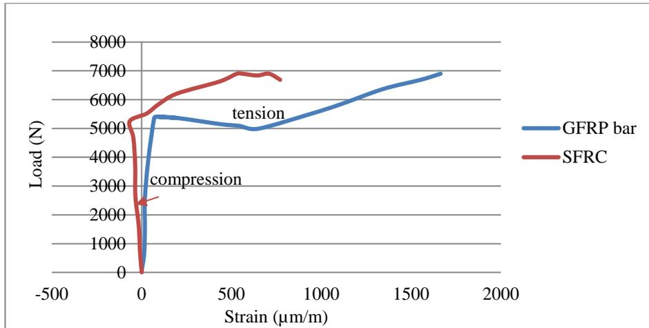
**Figure 5:** Load – strain curves of SFRC and GFRP bar
