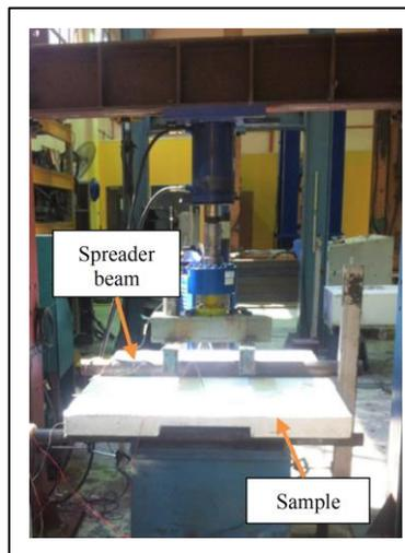
**Figure 3:** Sample tested under three-point load set-up
