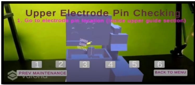
Fig. 6(a). The step-by-step procedure of the AR application for upper electrode pin checking.
