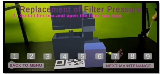
Fig. 5 (a). The step-by-step procedure of AR application for replacement of filter pressure.
