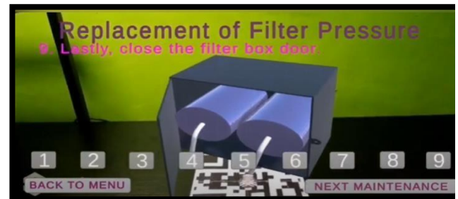
Fig. 5 (c). The step-by-step procedure of AR application for replacement of filter pressure.
