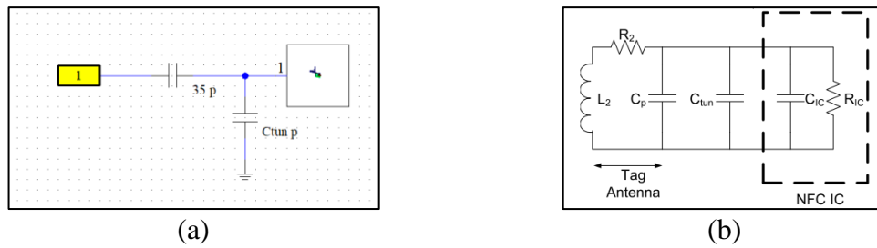
Figure 2: (a) Matching circuit in CST Design Studio and (b) equivalent circuit of NFC tag
