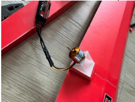
Figure 12. Electric Brushless Motor Attached to Wing
