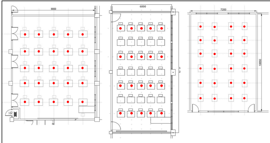
Figure 2: Position of points (a) Classroom 1 (b) Classroom 2 (c) Classroom
