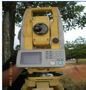
Figure 2. Total station used in establishing control points.
