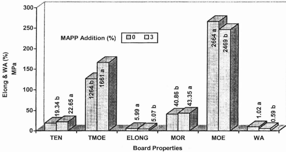
Figure 4: Effects of MAPP Addition on the Board Properties
