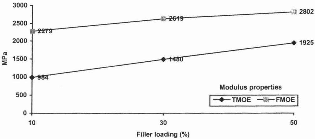
Figure 2. Effect of Filler Loading on the Tensile and Flexural Modulus
