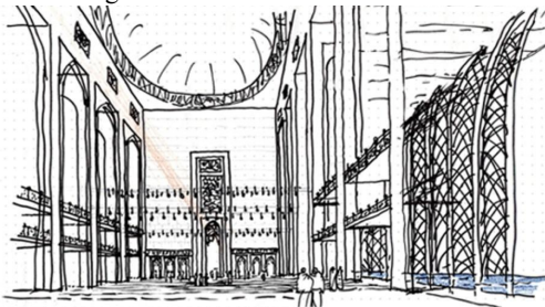
Figure 4. Sketches from the Architect show the design to provide cross ventilation and ample natural lighting to the buildings.
