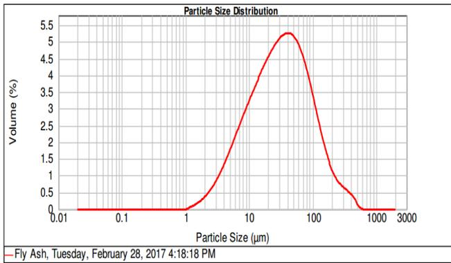
Fig. 1: Particle Distribution of fly ash sample.
