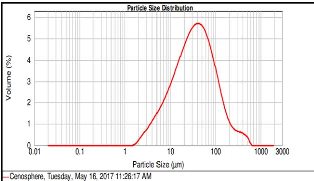
Figure 2 : Graph of Particle Distribution of Cenosphere sample.
