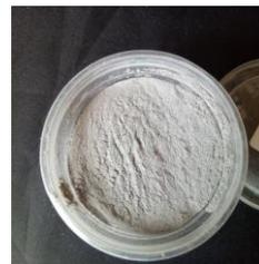
Figure 1 : Sample of coal fly ash that obtained from Kapar Power Plant.
