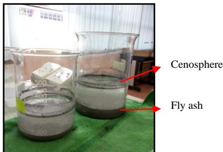
Figure 4 : Sedimentation process of sample.
