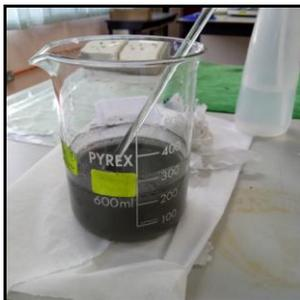
Figure 3 : Distilled water and fly ash were stirred for achieve complete mixture.
