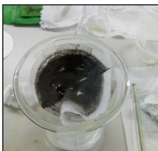
Figure 5: Portion of fly ash samples was skimmed and drained to ensure water content was eliminated.
