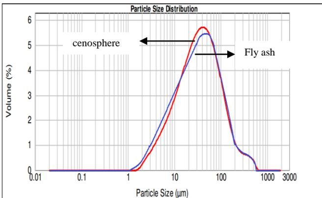
Figure 3 : Combination graph particle distribution of fly ash and cenosphere
