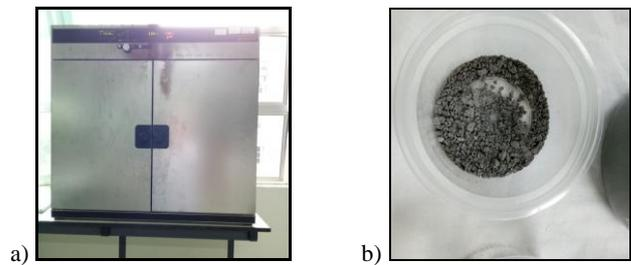
Figure 6 a and b: Sample of cenosphere undergoes drying process in an oven to eliminate moisture.
