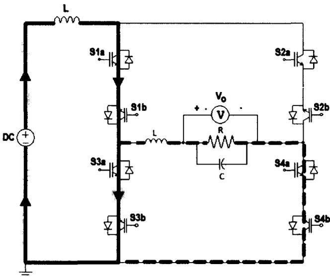
Figure 7: Positive cycle of boost inverter.
