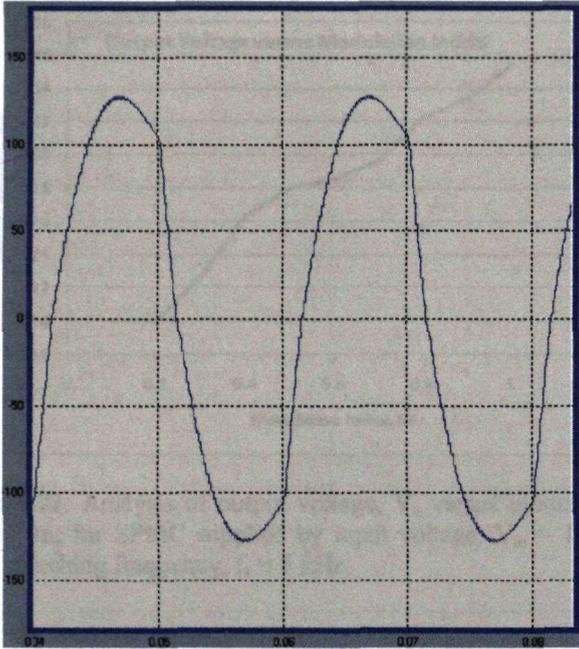
Figure 18: Simulation output voltage of R load (MLS) for modulation index,  $m_a = 0.7$ .
