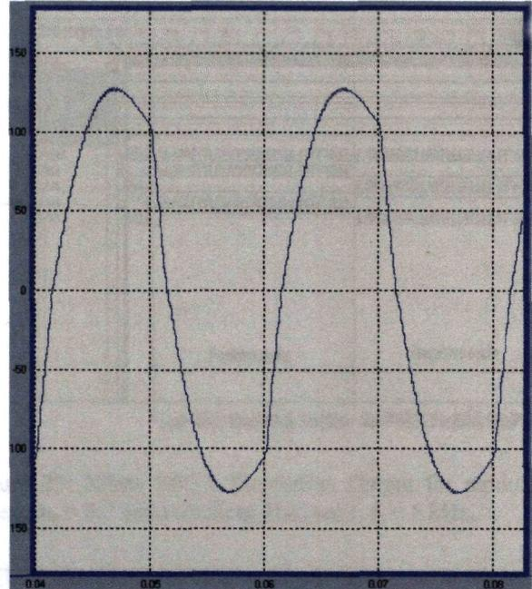
Figure 20: Simulation output voltage of R load (MLS) for modulation index,  $m_a = 1.0$ .
