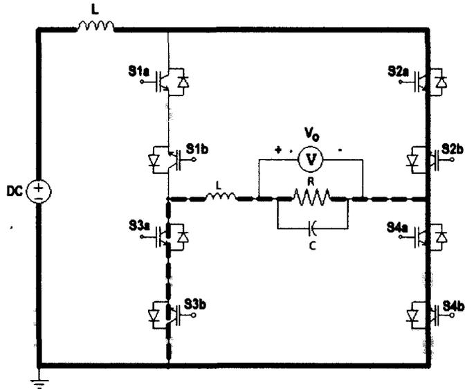
Figure 8: Negative cycle of boost inverter.
