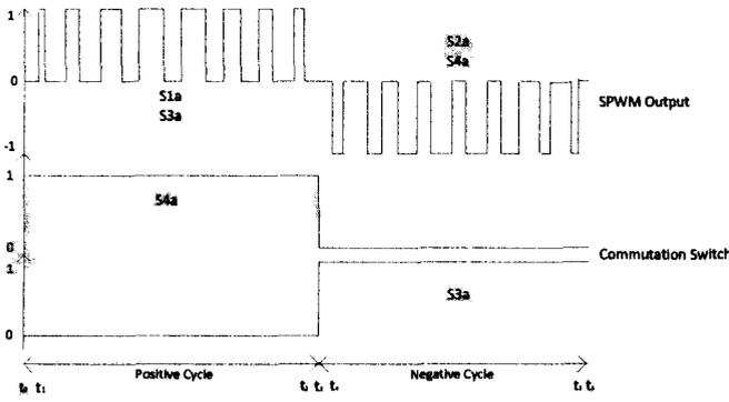
Figure 10: Switching pattern of boost inverter.
