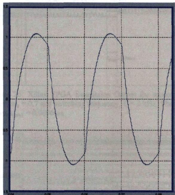
Figure 21: Simulation output current of R load (MLS) for modulation index,  $m_a = 1.0$ .
