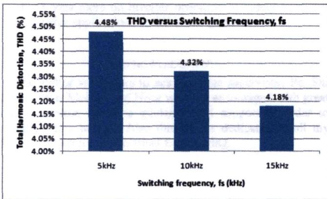
Figure 24: Total harmonic distortion, THD versus switching frequency,  $f_s$  for SPMC supplied by input voltage,  $V_{in} = 100$  V and modulation index,  $m_a = 0.7$ .
