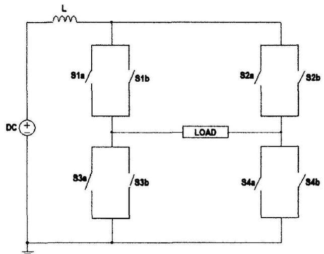
Figure 1: Single Phase Matrix Converter (SPMC) topology.
