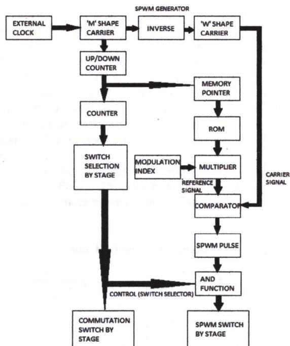
Figure 15: FPGA SPWM Generation Algorithm for Boost Inverter Operation.
