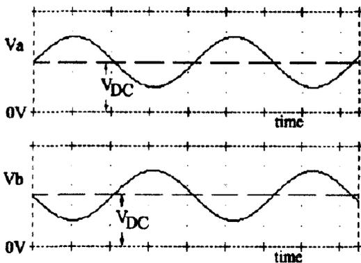
Figure 3: A basic approach to achieve dc-ac conversion, with boost characteristics.
