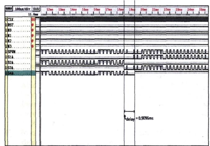
Figure 26: Xilinx FPGA Simulation Output for modulation index,  $m_a = 0.7$  and switching frequency,  $f_s = 3$  kHz. The time delay,  $t_{delay} = 0.9096$ ms.
