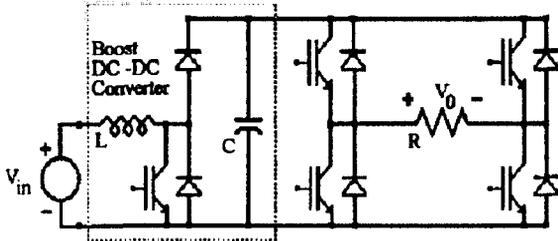
Figure 2: Circuit used to generate an ac voltage larger than the dc input voltage.
