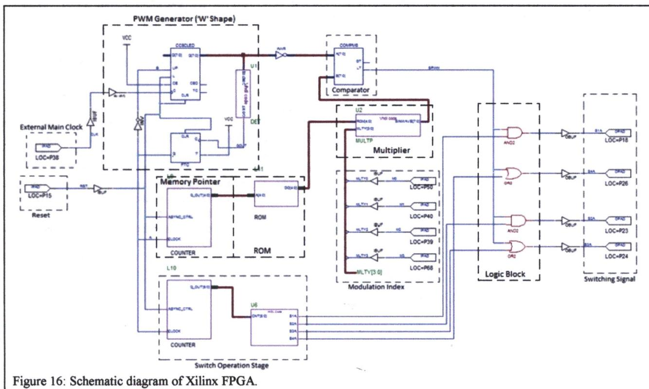
Figure 16: Schematic diagram of Xilinx FPGA.
