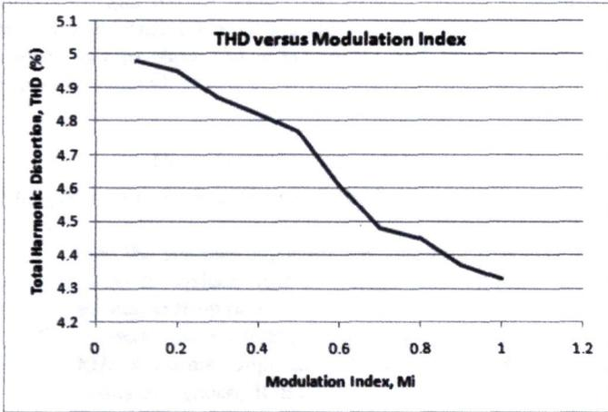
Figure 23: Total harmonic distortion, THD versus modulation index,  $m_a$  for SPMC supplied by input voltage,  $V_{in} = 100$  V and switching frequency,  $f_s = 5$  kHz.
