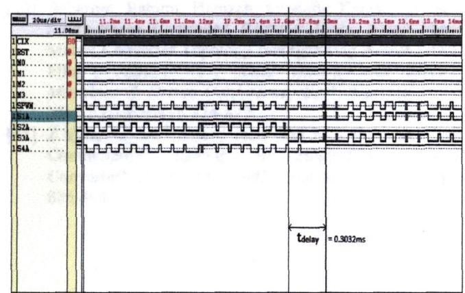
Figure 27: Xilinx FPGA Simulation Output for modulation index,  $m_a = 0.7$  and switching frequency,  $f_s = 6$  kHz. The time delay,  $t_{delay} = 0.3032$ ms.
