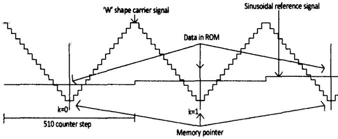
Figure 17: Illustration of memory pointer and data from ROM.
