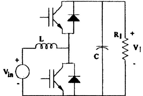
Figure 4: The current bidirectional boost dc-dc converter.
