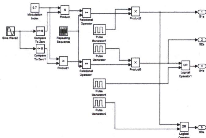
Figure 14: Controller unit for Boost Inverter.
