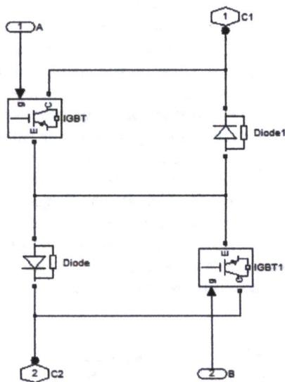
Figure 13: Bidirectional switches with diode pair.
