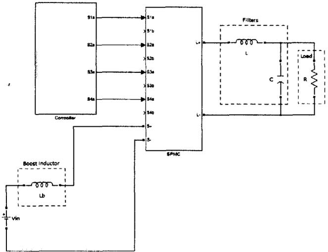
Figure 11: Modeling of Boost Inverter in MATLAB/Simulink.
