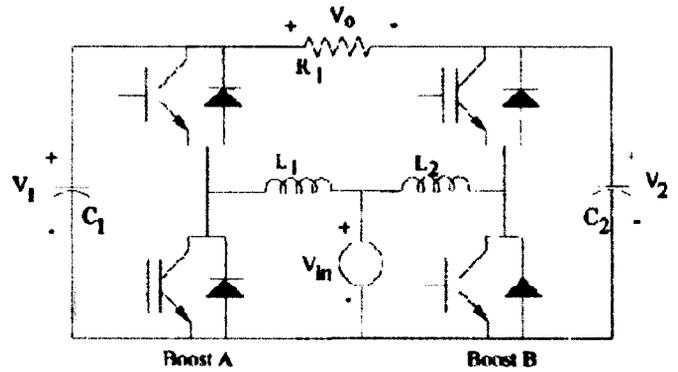
Figure 5: The dc-ac boost converter.
