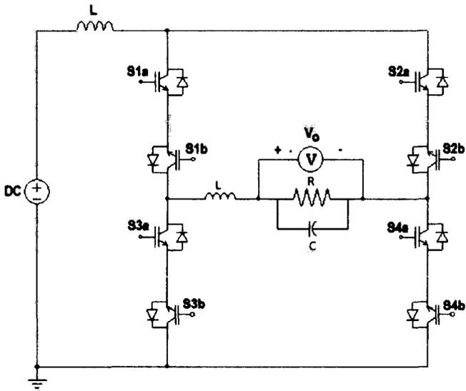
Figure 6: Proposed boost inverter using SPMC with LC filter.
