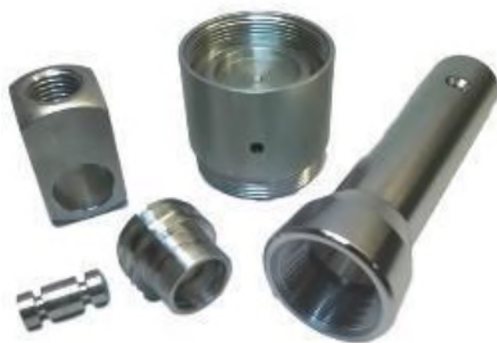
Figure 5: CNC Turning and Multi-Spindle Machining [26].
