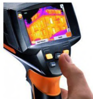
Figure 2: Non-contact temperature sensors
