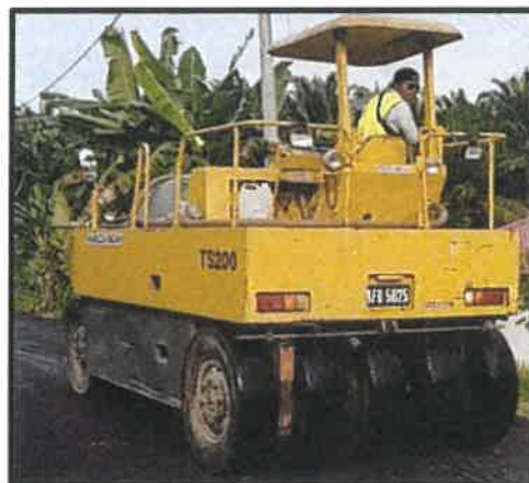
Figure 3.12 Pneumatic tyred roller
