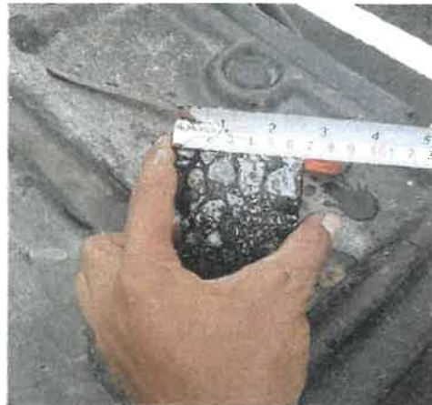
Figure 2.4 Measuring thickness of core sample
