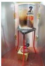
Figure 1. Sample are placed in the can for the slow pyrolysis process
