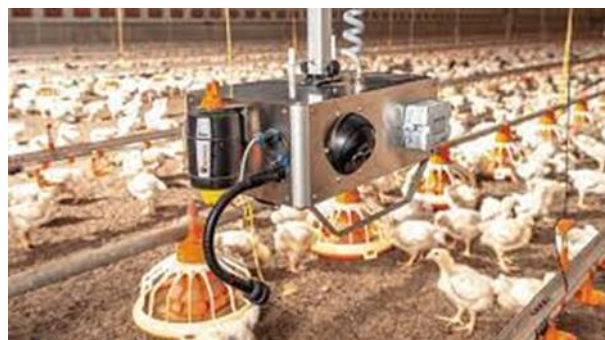
Figure 8: Chickenboy: The Smart Broiler Robot
