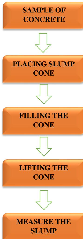
Figure 31: Methodology of Slump Test
