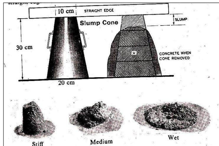
Figure 22: Type of Slump
