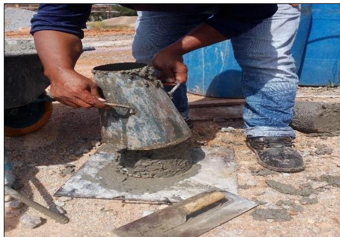
Figure 38: Lifting of Slump from Cone
