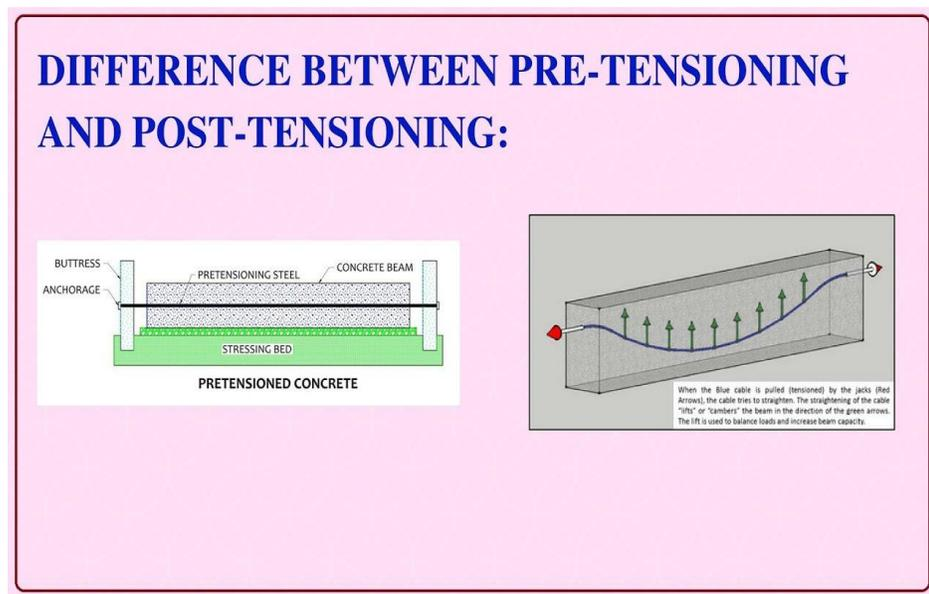
Figure 21: Difference between Pre-Tensioning and Post- Tensioning
