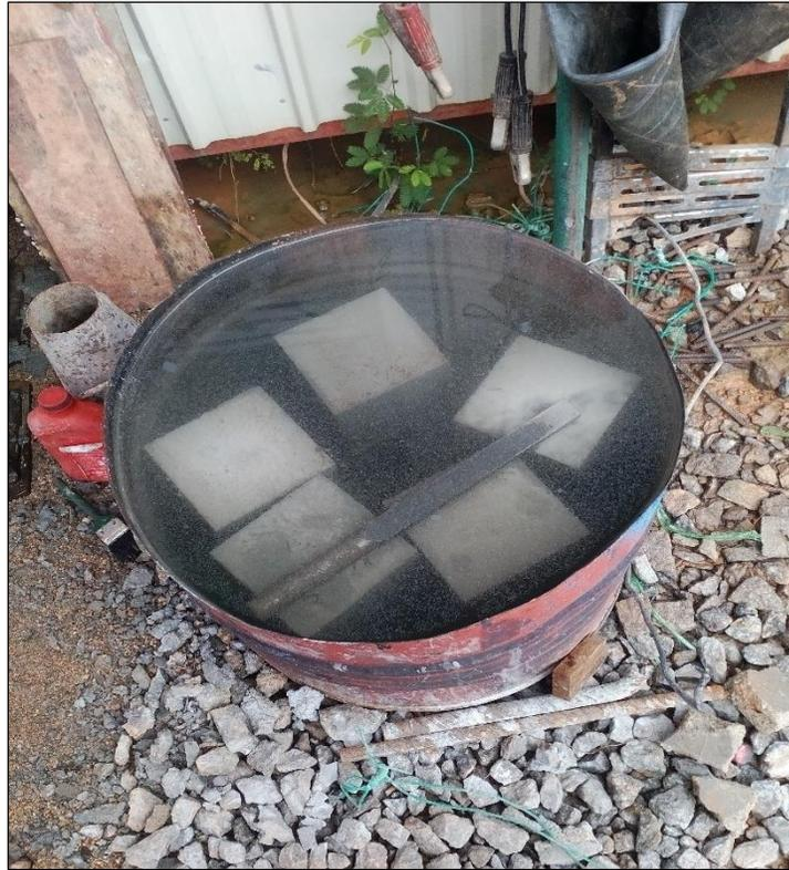
Figure 30: The Curing Process
