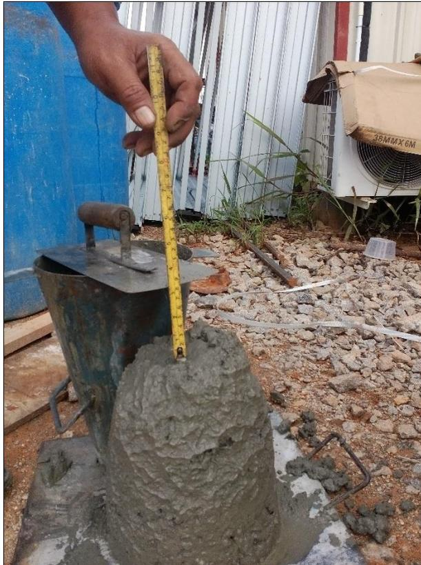
Figure 39: Measured of Slump Test
