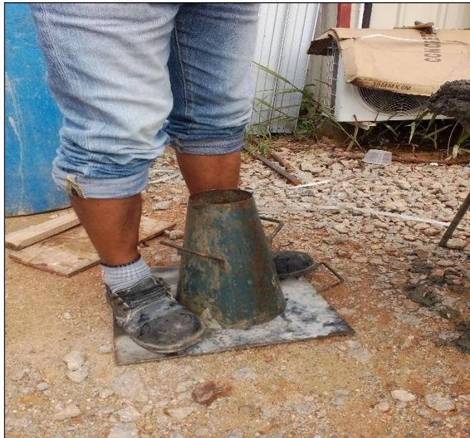
Figure 34: Placing the Slump Cone
