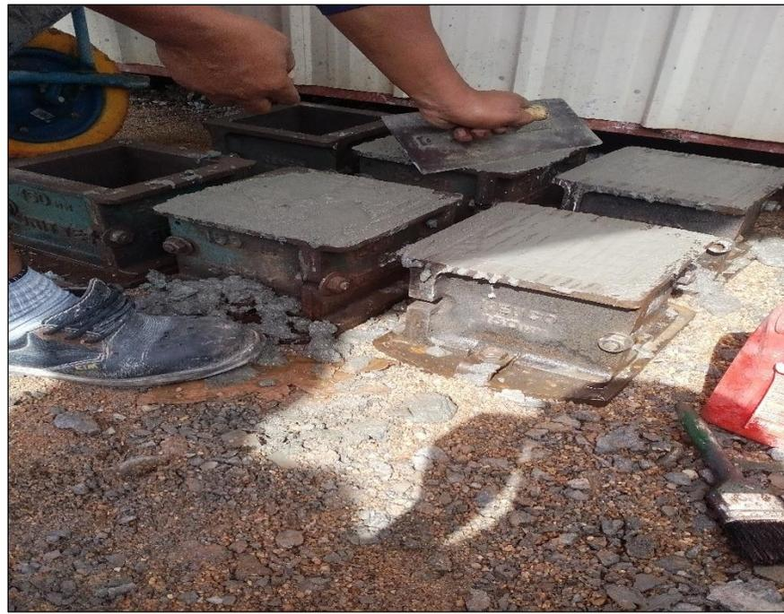
Figure 29: Level the Top Surface of Cube
