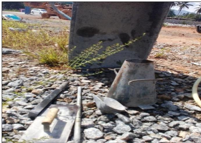
Figure 32: The Apparatus of Slump Test
