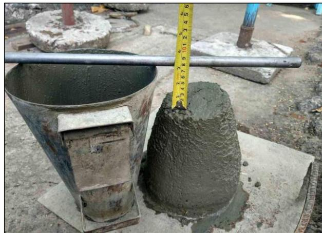
Figure 15: Slump Test
