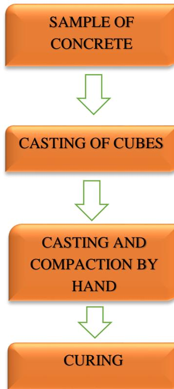
Figure 26: Methodology of Cube Test
