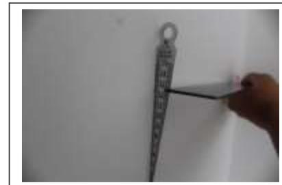
Wall squareness found misaligned and exceeded the tolerance of over 300mm
