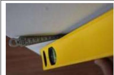
Wall found uneven and exceeded tolerance of 3mm over 1.2m (approximately 7.7mm)
