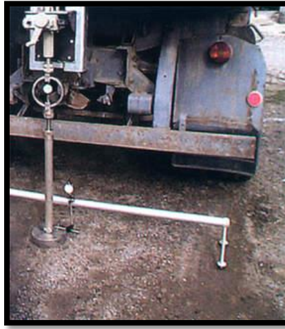
Figure 3.3 : The CBR equipment was installing at the lorry.
