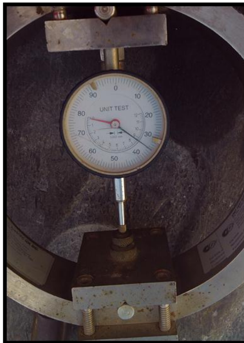
Figure 4.18 : Dial Gauge for penetration
