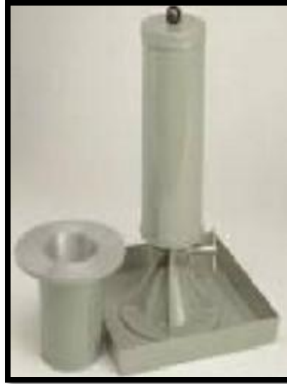
Figure 3.1 : Dynamic Cone Penetration Test and Tray Plate
