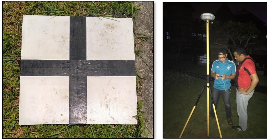
Figure 4: GCPs establishment; (Left) GCPs board marker and (Right) GCPs marking on the ground using MyRTKnet technique.
