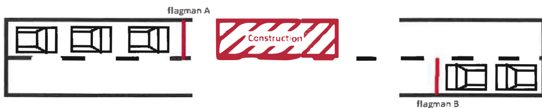
Figure 1.1 Visualization of two ways road under maintenance
