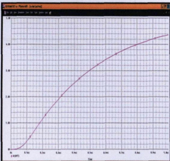
Figure 13: Output Voltage versus Elapsed Time (0.5Vdc)
