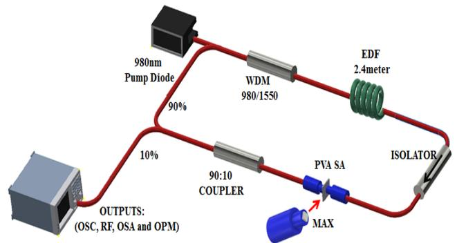
Fig. 3. Schematic diagram of the Q-switched fiber laser utilizing  $Ti_3AlC_2$  PVA as saturable absorber.
