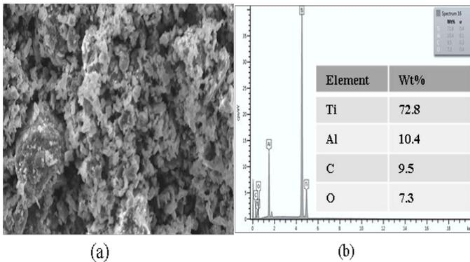
Fig. 1.Characteristics of  $Ti_3AlC_2$  film based saturable absorber (a) FESEM image (b) EDX analysis
