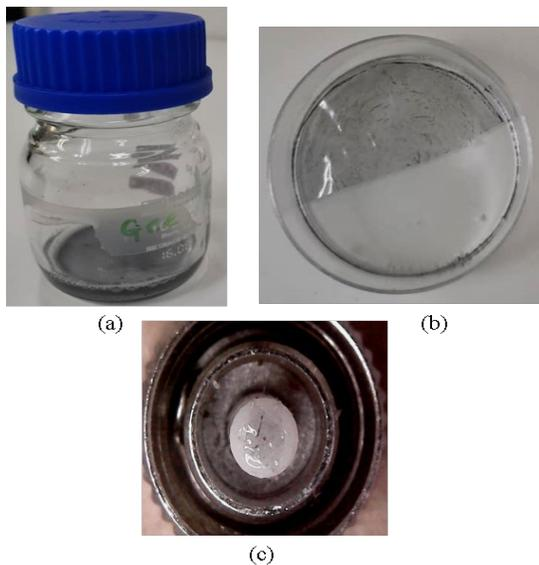
Fig. 2. Preparation of  $Ti_3AlC_2$  film based saturable absorber (a)  $Ti_3AlC_2$  solution that fully dissolved (b) peeling  $Ti_3AlC_2$  thin film that dried in a petri dish (c)  $Ti_3AlC_2$  film on the ferrule
