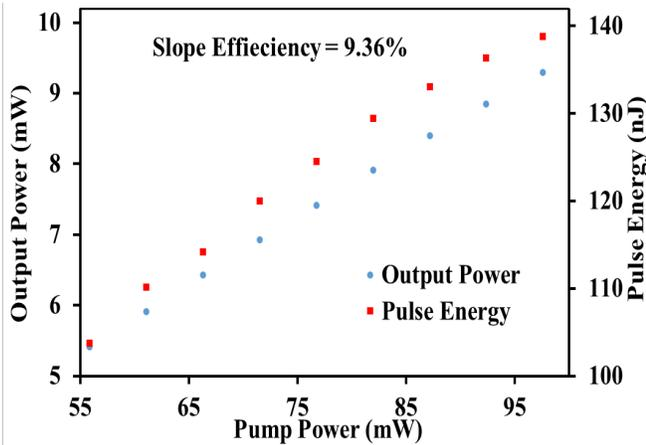
Fig 7. Output characteristics within 55.88mW to 97.62 mW of pump power of pulse energy and average output power.
