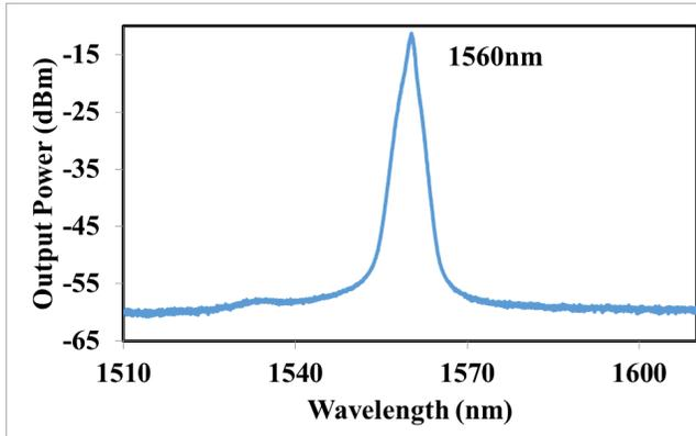
Fig 4. Output spectrum of Q-switched Ti<sub>3</sub>AlC<sub>2</sub> at pump power of 97.62mW
