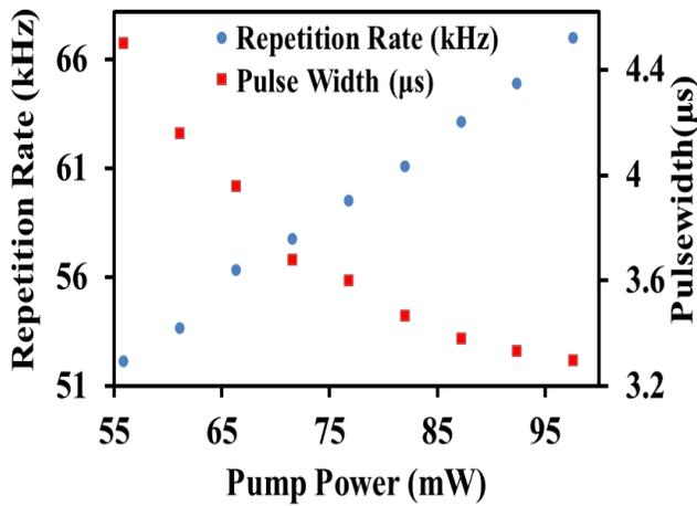
Fig 8. Output characteristics within 55.88mW to 97.62 mW of pump power: of repetition rate and pulsewidth
