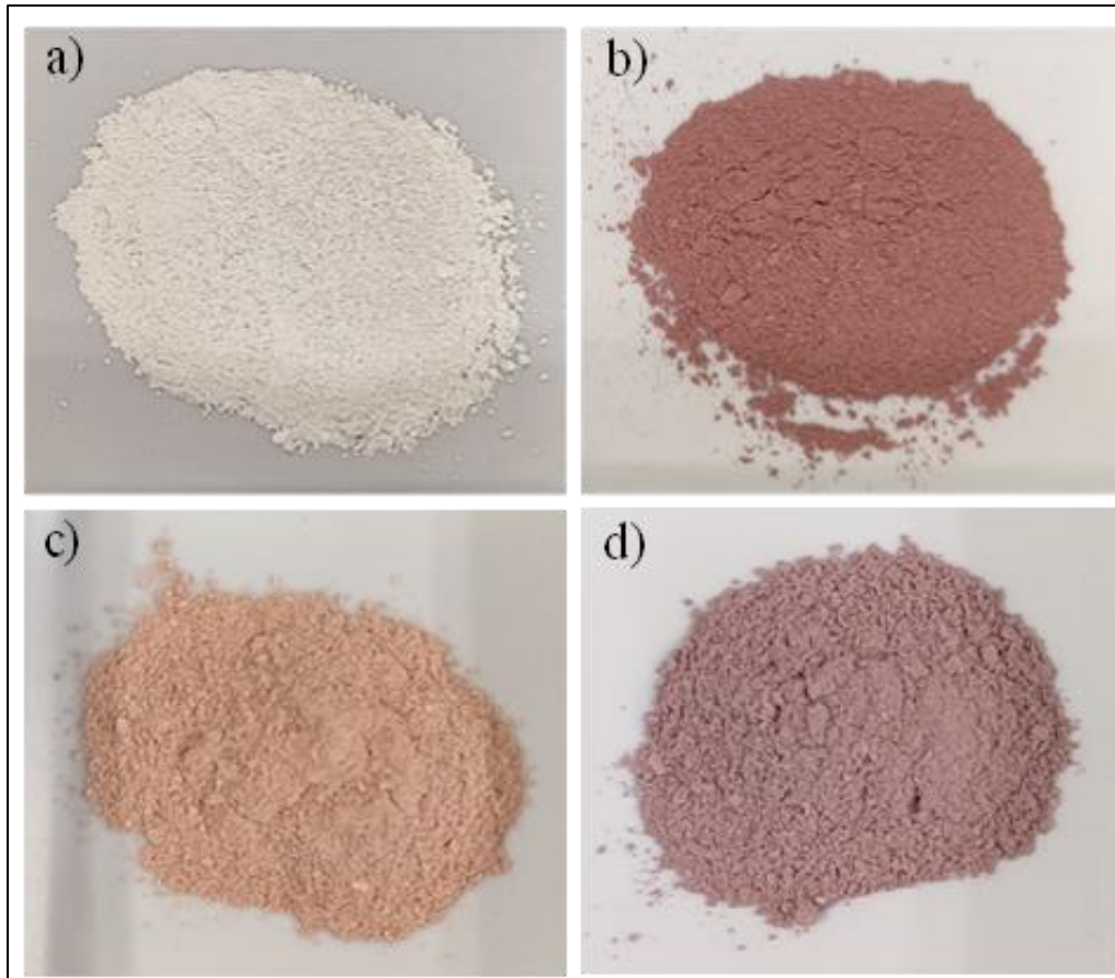
Figure 1: Colour intensity of photocatalyst of a) control, b) 1, c) 3, and d) 5 % Ag-TiO 2
