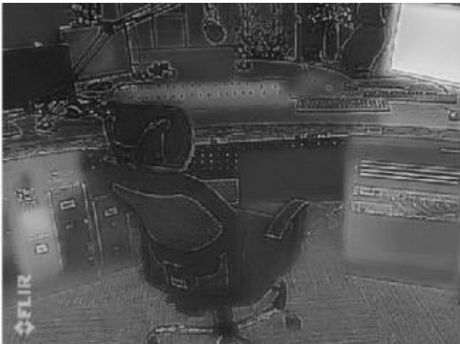
Fig. 9. Raw thermogram captured by FLiR One thermal camera.
