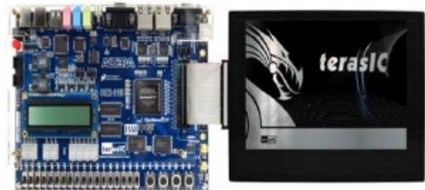
Figure 6. Hardware setup for interfacing MTL module with FPGA (DE2-115) board
