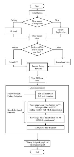
Fig. 3. The processing block diagram in Throb.
