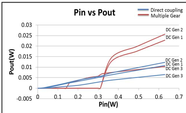
Fig. 14. Power input vs Power output of Direct coupling test and Multiple gear test
