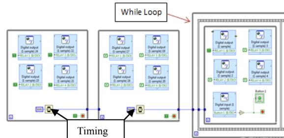
Fig. 8. Check all solenoid valves
