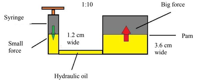
Fig. 3.Simple Hydraulic System
