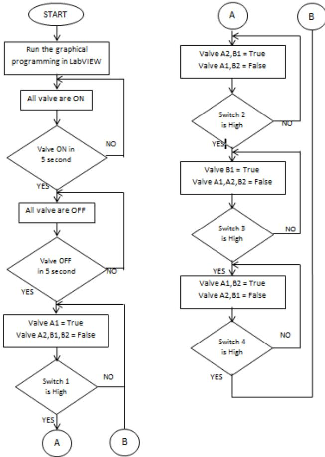
Fig. 7. The Flow chart of the controlled solenoid valve
