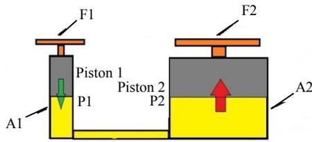
Fig. 4. The operation of hydraulic system
