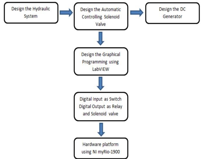
Fig. 6. Block Diagram of the Automatic Controlling System
