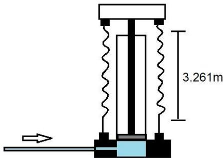
Fig. 5. The combination between hydraulic system and spring
