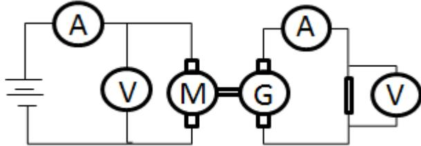
Fig. 10. Schematic diagram direct coupling
