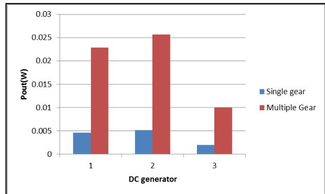
Fig. 15. Power output of implementation of DC generator with single and multiple gear implementation
