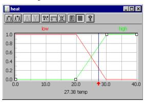
FIG. 4: The Fuzzy Input Variable 'Heat'
