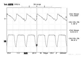
Fig. 9: Waveform of Output Sensor for Full Detection
