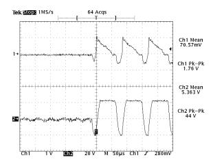
Fig. 8: Waveform of the Output Sensor Detecting a Human Presence
