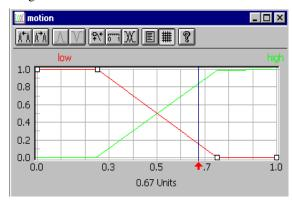
Fig. 5: The Fuzzy linput Variable 'Motion'
