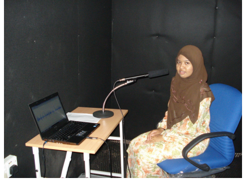
Fig. 1. Experimental setup for speech recording in semi-anechoic chamber.
