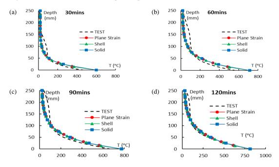
Figure 5: Temperature profiles of the one-way slab predicted by models built from different types of elements every 30 minutes.
