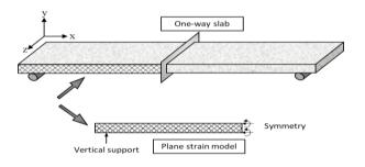
Figure 2: Development of Plane Strain Model
