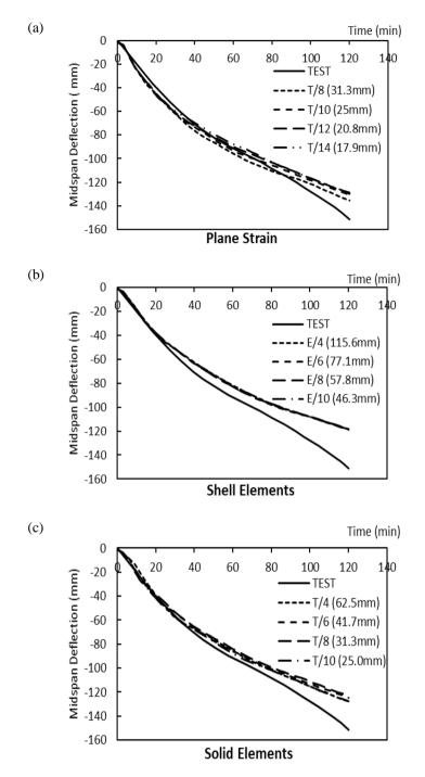
Figure 7: Midspan deflection response of a non-loaded 250mm one-way slab [1] from the model with different mesh sizes built from (a) plane strain model, (b) shell elements and (c) solid elements
