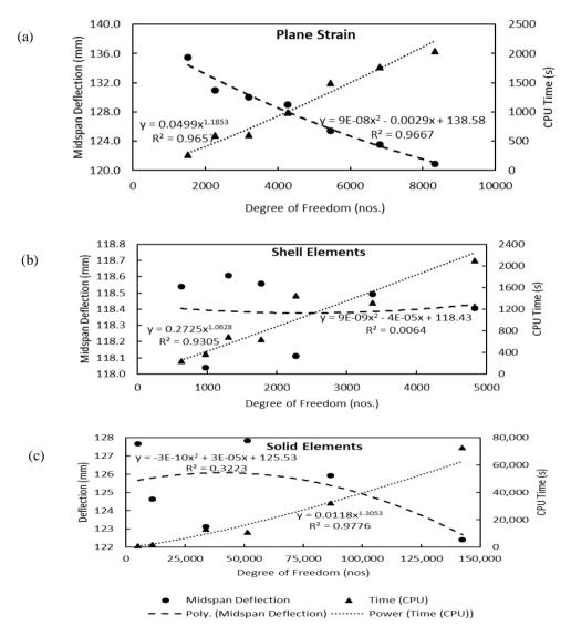
Figure 6: Relationship between the DOF numbers with midspan deflection and CPU time spend for analysis of non-loaded 250mm one-way slab build using (a) plane strain model, (b) shell elements and (c) solid elements.
