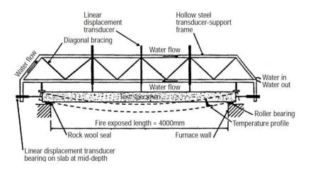
Figure 1: Experimental Arrangement of the One-Way Slab [1]
