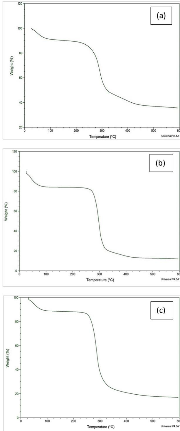
Figure 3: TGA curve for a) ACW/Fe<sub>2</sub>O<sub>3</sub>, b) ACW/NiO, and c) ACW/Al<sub>2</sub>O<sub>3</sub> NPs adsorbents
