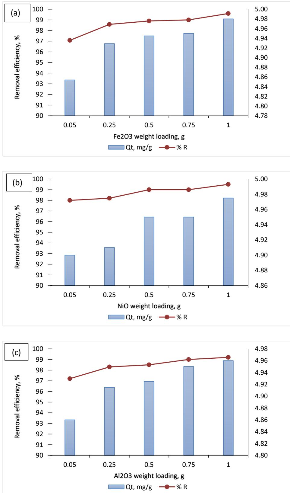
Figure 2: Effects of a) ACW/Fe<sub>2</sub>O<sub>3</sub>, b) ACW/NiO, and c) ACW/Al<sub>2</sub>O<sub>3</sub> NPs adsorbents at different weight loadings toward Pb<sup>2+</sup> removal
