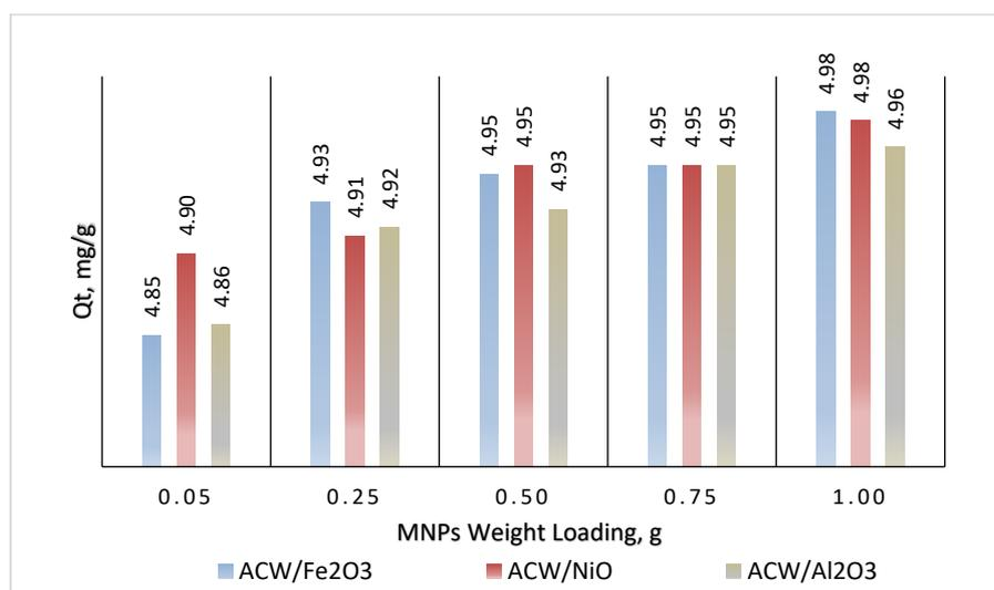
Figure 1: Effect of different types of MNPs modified on ACW toward Pb<sup>2+</sup> removal
