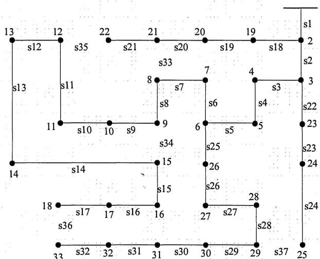
Figure 5: Initial configuration of 33-bus distribution system
