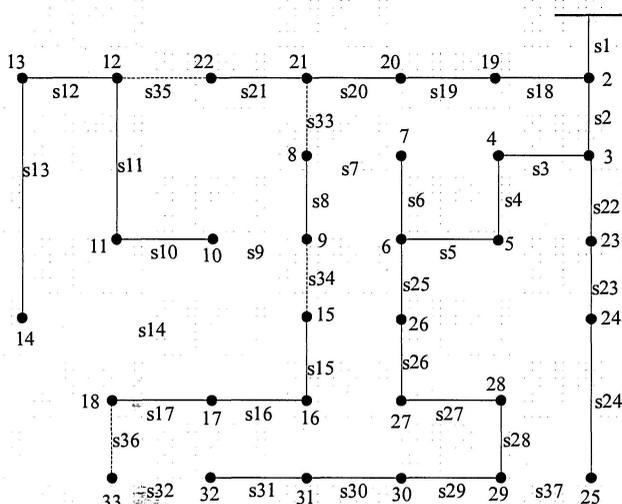
Figure 7: Second stage configuration of 33-bus distribution system
