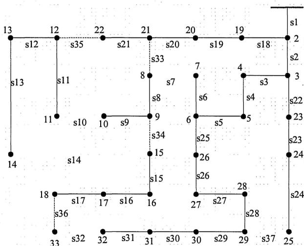
Figure 6: First stage configuration of 33-bus distribution system
