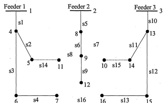
Figure 4: Final configuration of 16-bus system
