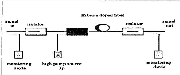
Figure 1: Forward pump EDFA setup
