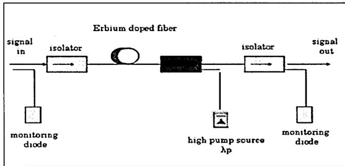
Figure 2: Backward pump EDFA setup
