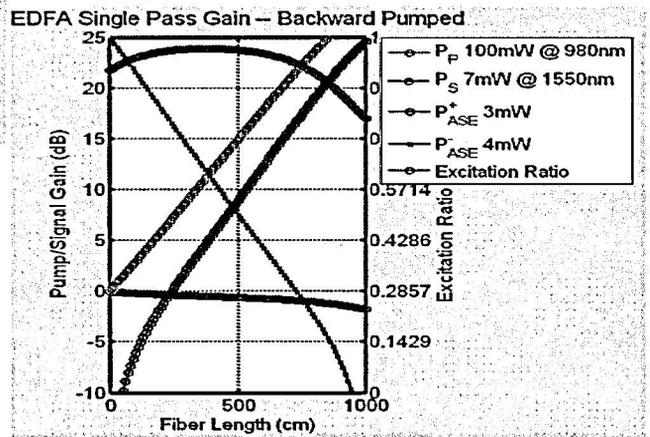
Figure 12: EDFA Single Pass Gain backward pump
