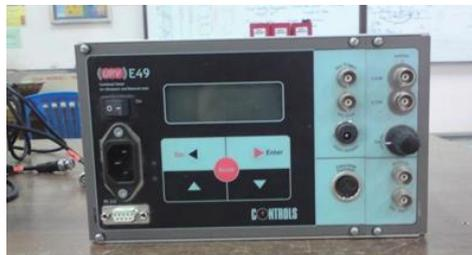
Figure 5: P-wave instrument (UPV)
