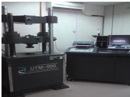
Figure 7: Universal Testing Machine (UTM 500)
