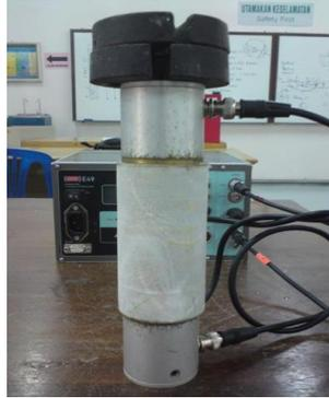
Figure 6: The sample was connected to the UPV
