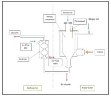
**Fig. 1** Schematic diagram of bio-oil produced via fast pyrolysi
