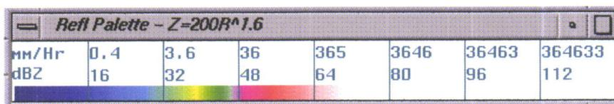
Figure 6: Weather radar precipitation color palettes (MMD,2003)
