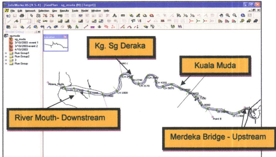
Figure 8: Muda River Hydrodynamic Model for Input from Weather Radar
