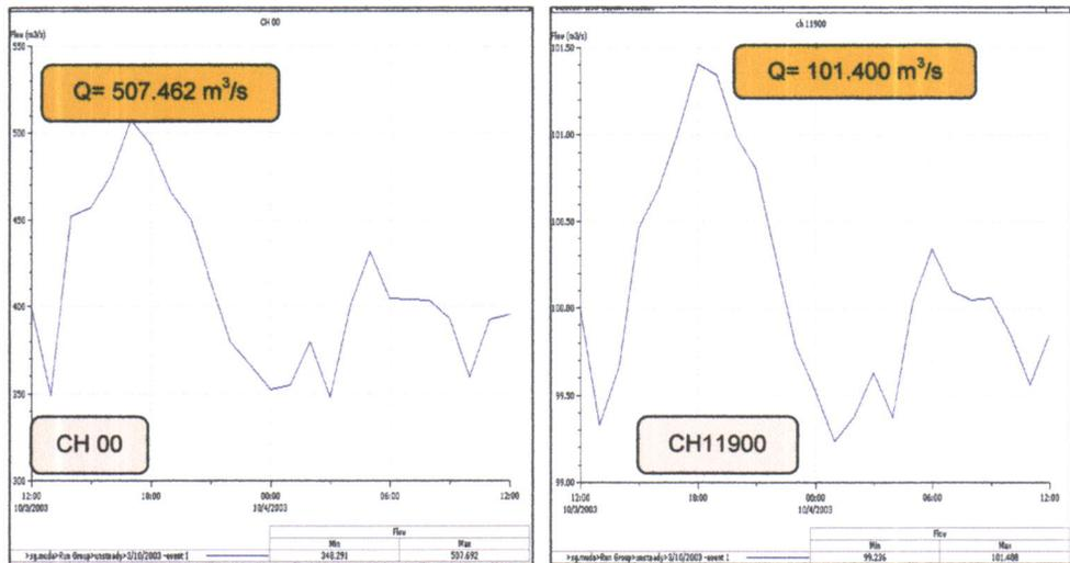
Figure 10: Flow Hydrograph at CH 00 and CH 11900
