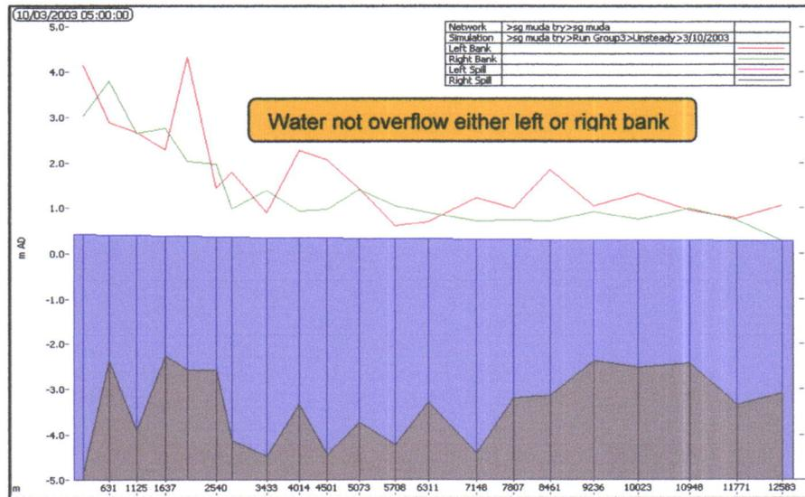
Figure 11: Longitudinal Cross Sections (3<sup>rd</sup> October 2003 event)
