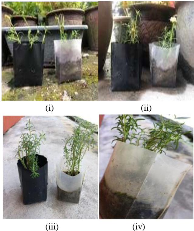
Fig. 2: Photograph of LDPE-CS bag (right-white) and commercial polybag (left-black): (i) day 1, (ii) day 5, (iii) day 60, (iv) small hole spots of LDPE-CS after day 60.
