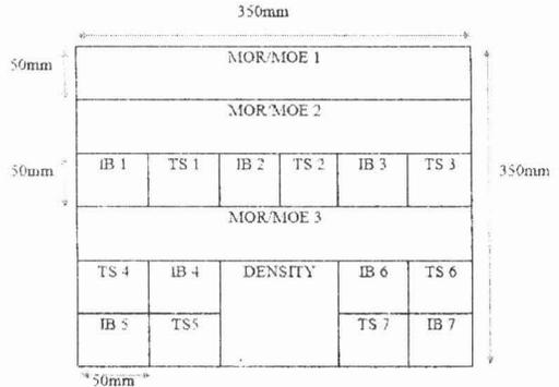
Note: MOR= Modulus of rupture, MOE= Modulus of elasticity, IB= Internal bonding, TS= Thickness swelling
