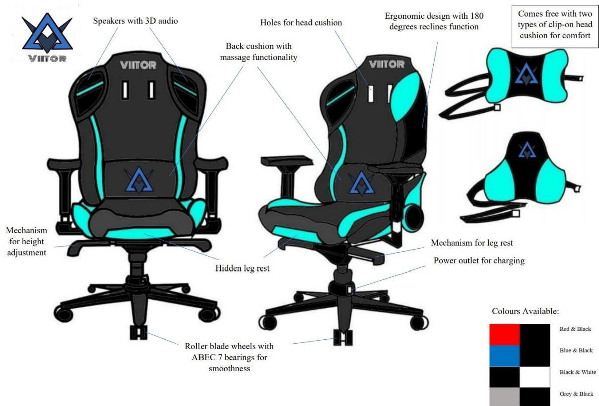
Figure 2.4: Specifications Diagram for Viitor Gaming Chair
