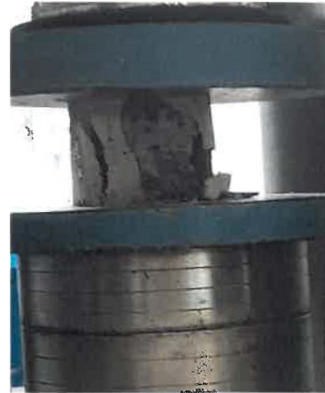
Figure 2.2: The brick after failure
