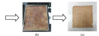
Fig. 2. (a) Preparation of materials; (b) Preparation of banana paper; (c) Banana fibre paper.
