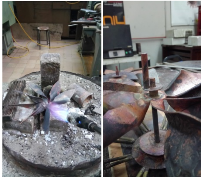
Figure 8. Anneal and solder all parts
